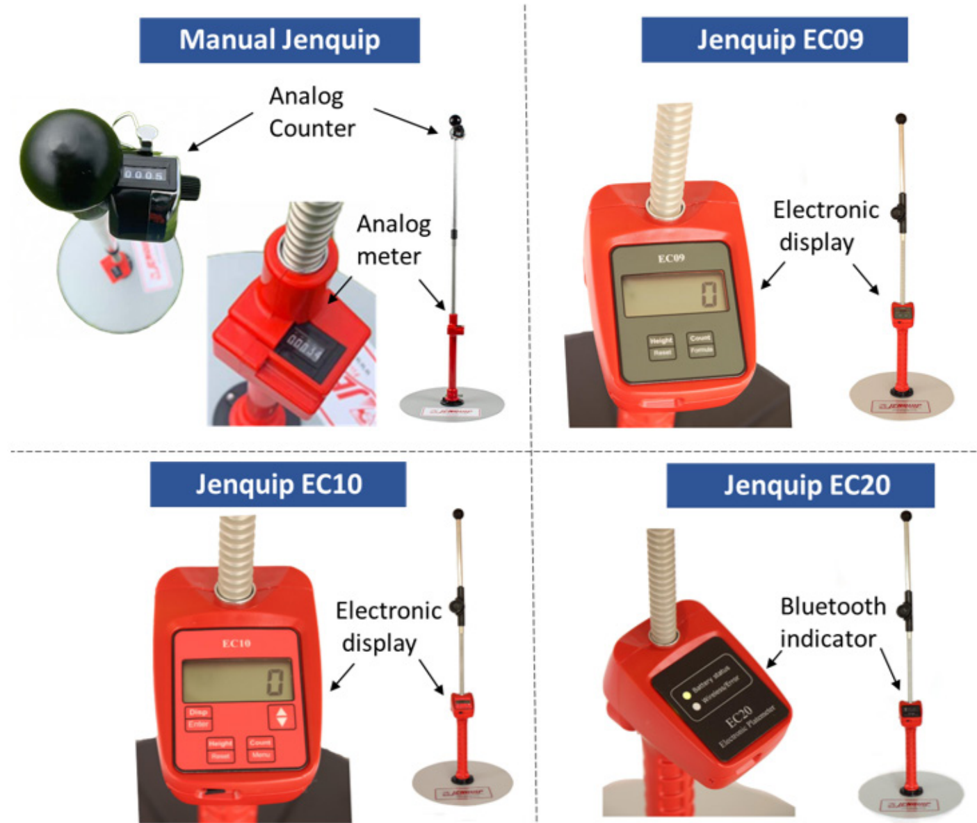
Figure 3: Examples of models of RPMs commercially available in North America. Each model has different functions for data collection, data storage and forage calculation. The Manual Jenquip (top left) requires that producers take note of each measurement in the field from the analog meter and counter, and manually calculate the available forage in each paddock. The Jenquip EC09 (top right) automatically calculates available forage in each paddock (shown in the electronic display), but still requires that producers take note of each measurement in the field since the data cannot be automatically saved. The Jenquip EC10 (bottom left) automatically calculates available forage in each paddock (shown in the electronic display) and stores data for up to 99 paddocks, which can be later downloaded via USB cable. The Jenquip EC20 (bottom right) automatically calculates available forage and stores the data on the user's smartphone (either Android or iOS) via Bluetooth connection. The Jenquip EC20 also collects and saves the GPS location for each measurement taken. To our knowledge, only RPMs manufactured by Jenquip (NZ-based) are commercially available in North America. Other options available elsewhere include Platimeters™ (NZ-based) and Grasshopper (UK-based).
