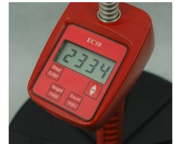
Figure 5: Example of how the amount of available forage is shown on the display of the RPM Jenquip EC-10. Depending on how it is configured, the display represents the available forage per paddock (DM lbs/paddock) or per acre (DM lbs/acre).
